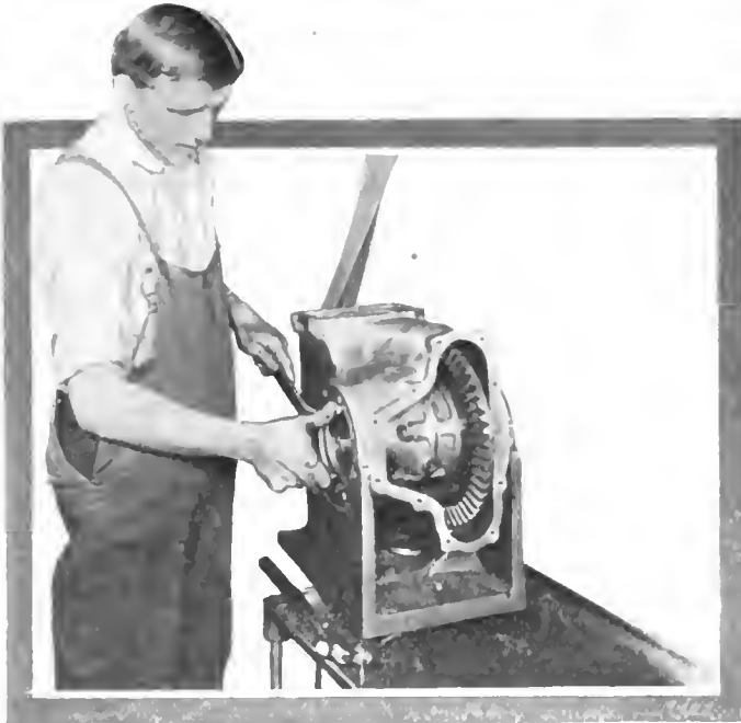
Some of the manufacturing operations which are most expensive, both in time and money, are those little steps toward the perfected mechanism which are least in the limelight. The picture shows a workman adjusting the bearing in the differential of a White 1.5-ton truck so that the gears will mesh perfectly when the parts are assembled.
